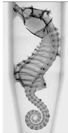
▲ DELab \mu CT-100X Dwarf seahorse, 40 kVp, resolution: 7.5 \mu m A combination of 2D and 3D images shows the characteristics of the seahorse, including the interior and exterior, biological features, structure, and number of bones.
