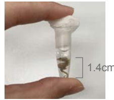
▲ DELab \mu CT-100X Dwarf seahorse, 40 kVp, resolution: 7.5 \mu m A combination of 2D and 3D images shows the characteristics of the seahorse, including the interior and exterior, biological features, structure, and number of bones.
