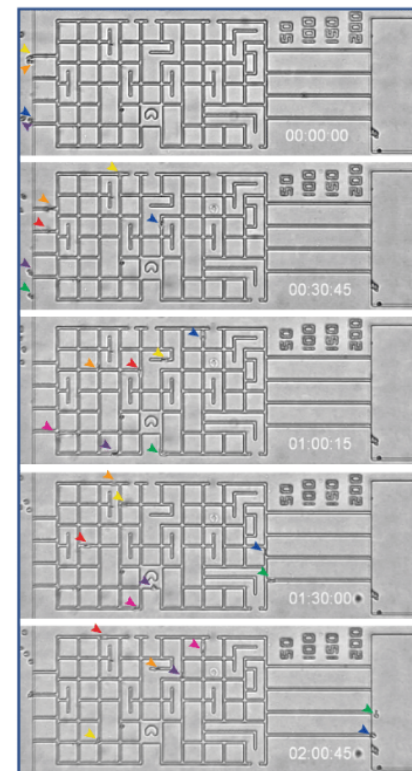
Fig. 3. Human neutrophils navigate their way through a microscopic size maze (total maze size is 0.8 mm) towards a reservoir with chemoattractant on the right. Colored arrowheads indicate the same neutrophils at different timepoints. The speed and directionality of neutrophil movement towards the chemoattractant is followed using the CytoSMART® Lux2.
