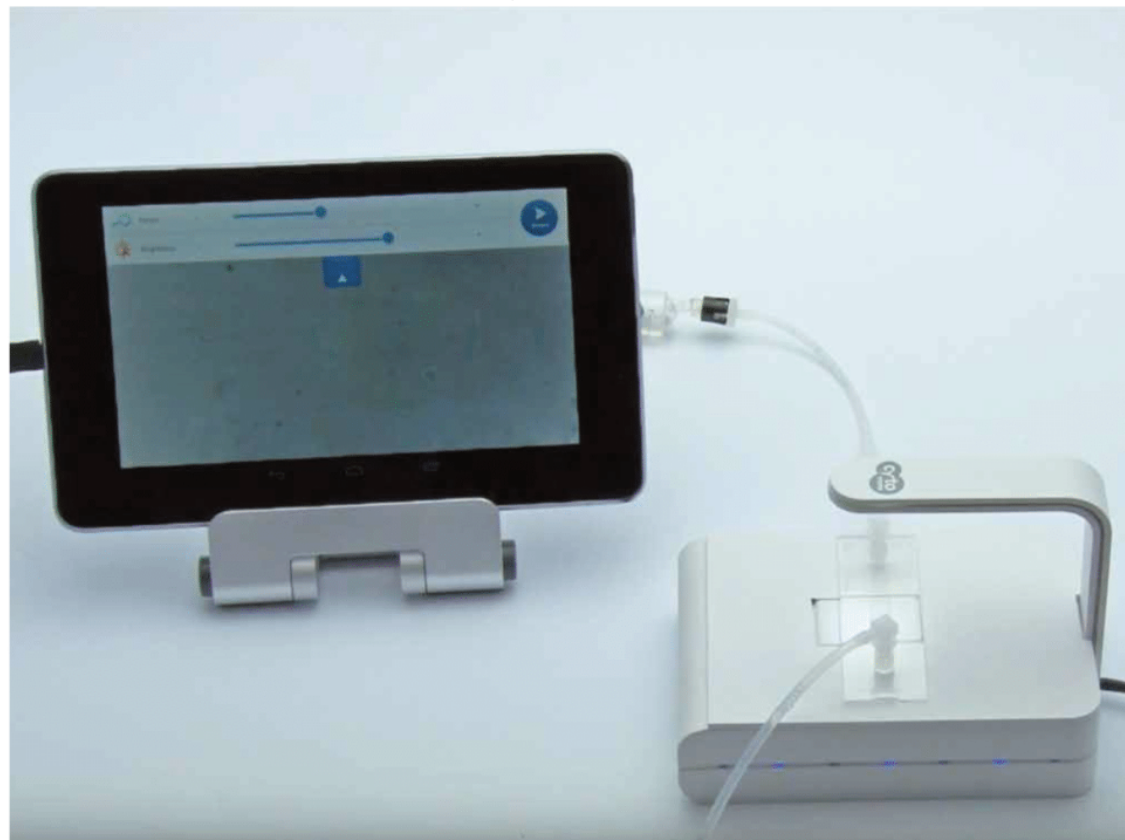
Figure 5. The open design of the CytoSMART™ Lux2 enables easy monitoring of cells cultured inside microfluidic devices. In this case, the flow and attachment of cells within a microfluidic chip is monitored.
