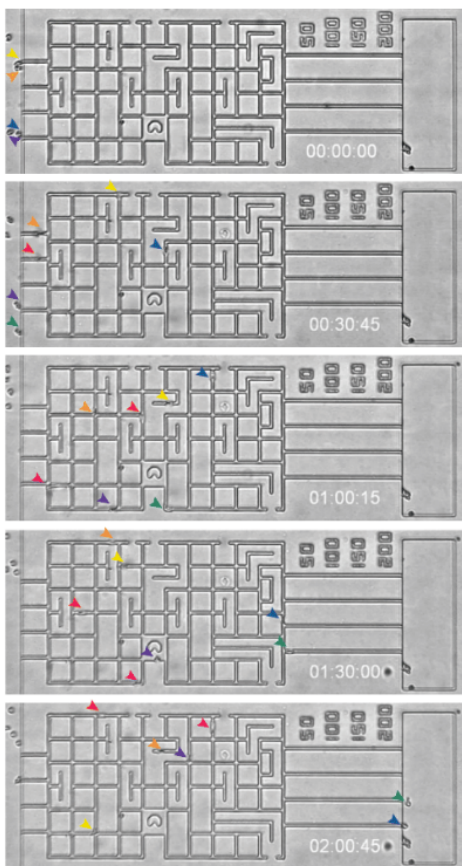
Figure 4. Human neutrophils navigate their way through a microscopic size maze (total maze size is 0.8 mm) towards a reservoir with chemoattractant on the right. Colored arrowheads indicate the same neutrophil at different timepoints. The speed and directionality of neutrophil movement towards the chemoattractant is followed using the CytoSMART™ Lux2.
